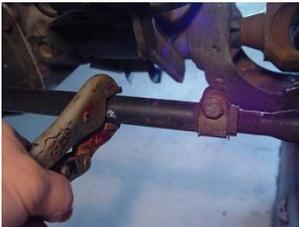
**3.** Grab the tie-rod with a pair of vice-grips or pipe wrench and rotate it a little bit at a time taking measurements along the way. Continue this process until the width in the front is about 1/16" (but no more than 1/8") closer together than the back.
