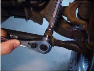
**2.** Using a 13mm socket and wrench, loosen sleeves on both ends of the tie-rod.
